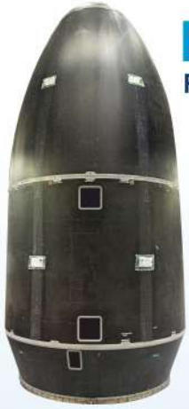
5m Ø 10.7m Height Payload Fairing Assembly for GSLV Mk-III
