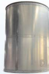
2m Ø Metallic Sandwich Structure for SSLV
