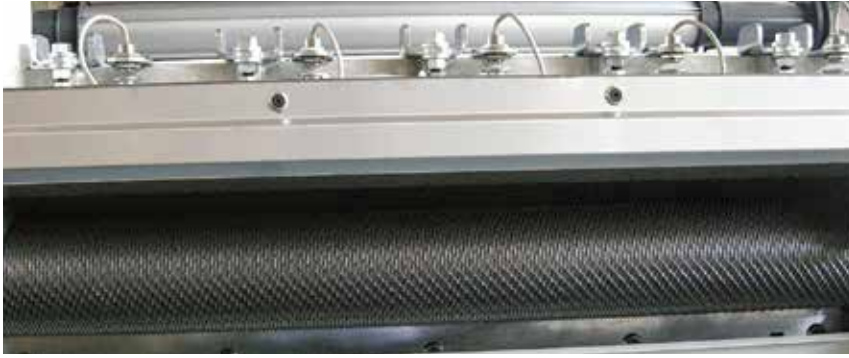
Five Level Sensor Arrangement
